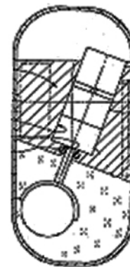
Fig. (14). Representation of the capsule with ultrasonic module described by the invention of Taniguchi.
