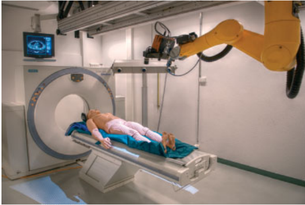
Figure 1. Virtobot set-up with CT scanner, Virtobot with mounted surface scanner and Optotrak tracking system in the background
